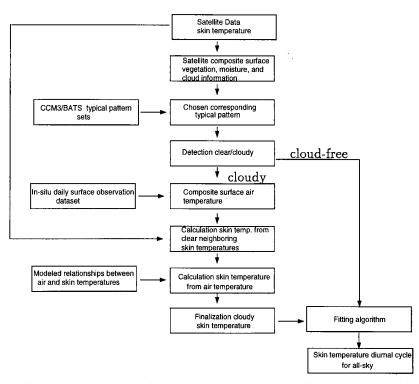
Figure 2. Flow diagram showing the major steps of the land surface diurnal cycle algorithm. See text for details.
