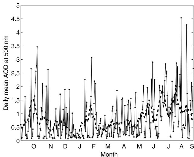
**Figure 1.** Daily mean aerosol optical depths measured by a Cimel Sun photometer from October 2004 to September 2005 at the Xianghe site. The dashed curve shows the 10-day running averages of the AOD.
