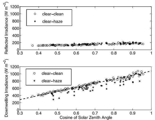
**Figure 9.** Solar irradiance (top) reflected at the top of the atmosphere (from the CERES SSF product) and (bottom) incoming on the ground (measured) for clear-clean (AOD < 0.2) and clear-hazy conditions (AOD > 0.2).
