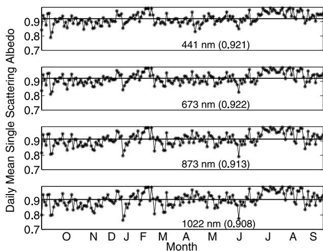
**Figure 5.** Daily mean single scattering albedos (corresponding to AOD at 440 nm > 0.4) retrieved from the Cimel sky radiances at 441, 673, 873 and 1022 nm. Data are from September 2004 to September 2005. Overall average at each wavelength is in parentheses.
